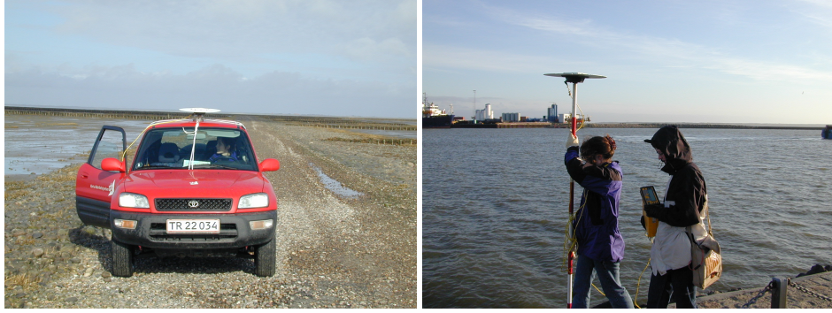
Figure 4.2: To validate the DEM, GPS control points were collected. This was done with a roof-mounted antenna on a car (left) and by moving the antenna around Esbjerg harbour by foot (right).
