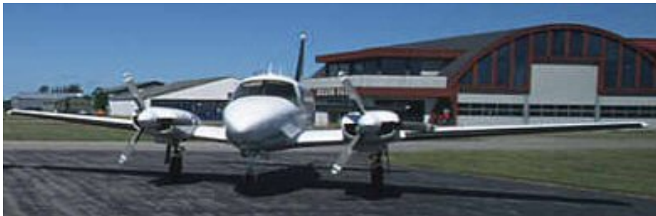
Figure 2.1: The twin piston engine Navajo PA 31 (OY-BHF) that served as platform for the LiDAR system, was chartered from the Danish surveying company, Scankort.
