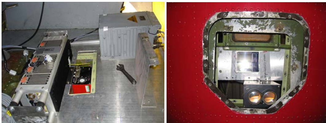
Fig. 5.4 Riegl laser scanner mounted in the aircraft (left) and aircraft hole photographed from under, with scanner mirror, and camera (right).
