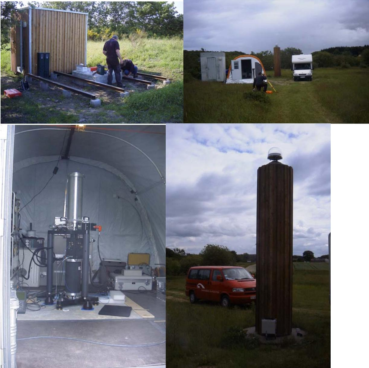
**Figure 1.** The absolute gravity campaign in Denmark 2005. (top left) Suldrup absolute gravity station: fixing the iron girders outside the hut to support the wooden floor of the tent; (top right) Smidstrup absolute gravity station: the weatherport; (bottom left) Smidstrup absolute gravity station: FG5 # 220 of the Institut für Erdmessung, Hannover, inside the tent; (bottom right) Smidstrup absolute gravity station: eccentric point at the foot of GPS-antenna measured using Scintrex CG3 of IfE.
