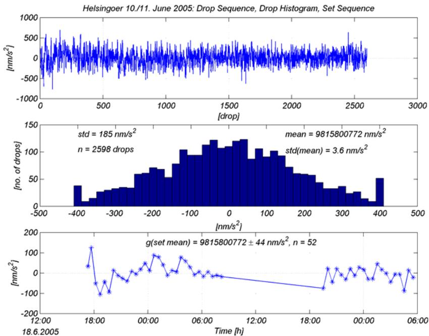
**Figure 3.** Some details concerning the 2005 gravity measurements in Helsingør. (1 set=50 drops).
