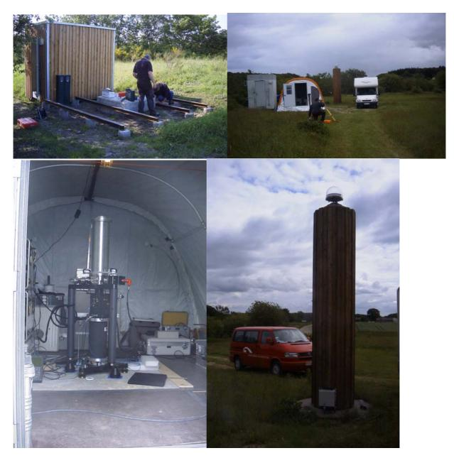
**Figure 1.** The absolute gravity campaign in Denmark 2005. (top left) Suldrup absolute gravity station: fixing the iron girders outside the hut to support the wooden floor of the tent; (top right) Smidstrup absolute gravity station: the wheatherport; (bottom left) Smidstrup absolute gravity station: FG5 # 220 of the Institut für Erdmessung, Hannover, inside the tent; (bottom left) Smidstrup absolute gravity station: eccenter point at the foot of GPS-antenna measured using Scintrex CG3 of IfE.
